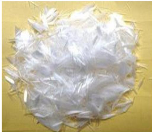
**Fig. 4.** Multifilament polypropylene fibers
